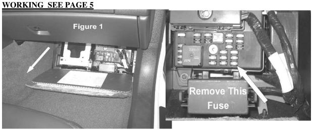
Insert the new fuse adapter into the slot you just removed the 10A fuse from. The adapter must be installed as shown with the white wire facing up and the red wire facing the center console. Remove the grounding screw, and re-install it with the two black ground wires by inserting the screw through the connector, tighten. Slip the control box into the location shown and place the blue antenna wire tucking it into the space shown (see fig. 2)
