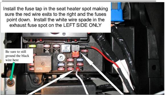
Install the white wire spade in the exhaust fuse spot on the LEFT SIDE ONLY
